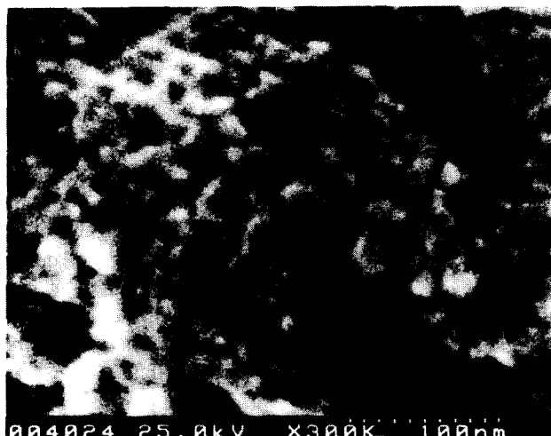
Fig. 4. SEM photograph showing the surface morphology of a TiO 2 film prepared by heating at 450 °C for 30 min.
